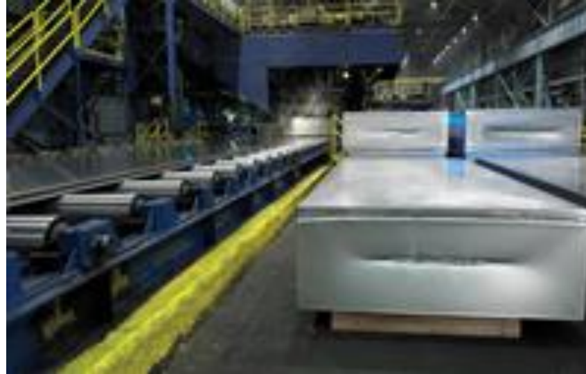
Scalped rolling slab ready for hot mill
