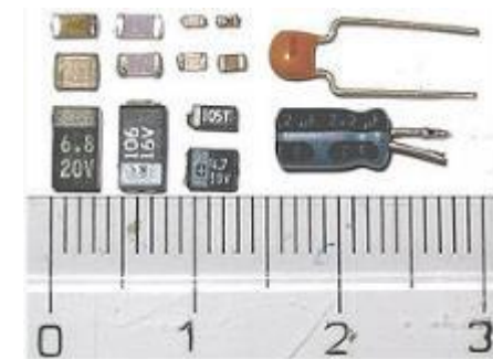
Miniature low-voltage capacitors (next to a cm ruler)
