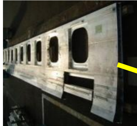
Shinkansen side panel extrusion profile
