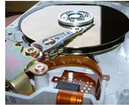
Inside view of a hard disk
