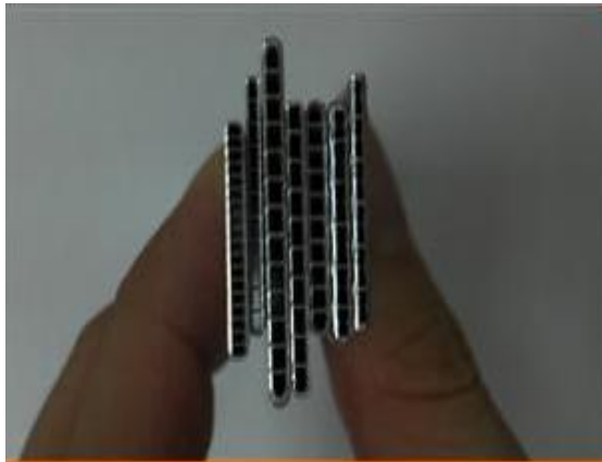
Multiport condenser tubing for air conditioners
