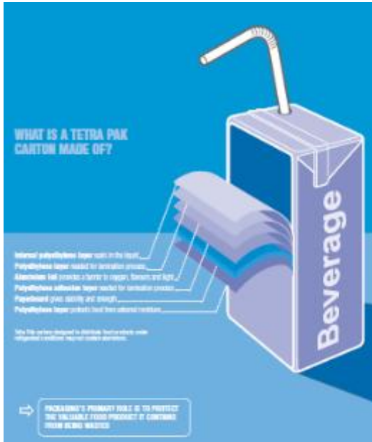
Light gauge (6 micron) Tetrapak foil
